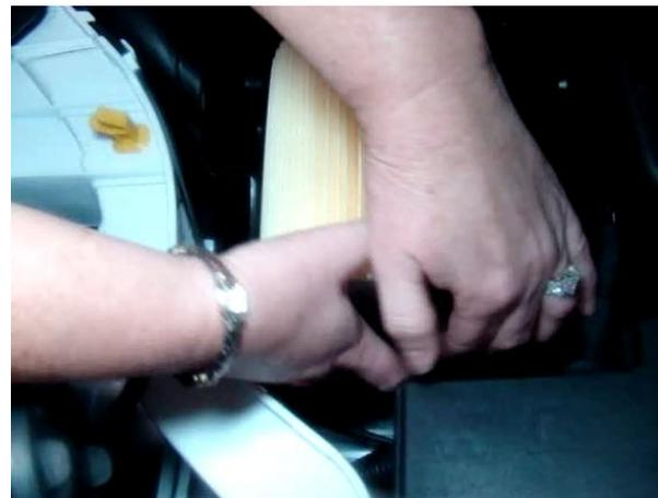
Figure 6: Seat closed end of Filter in housing
